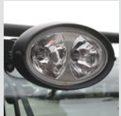
2 x Dual Power working lamp front, 1 x Single Power rear
