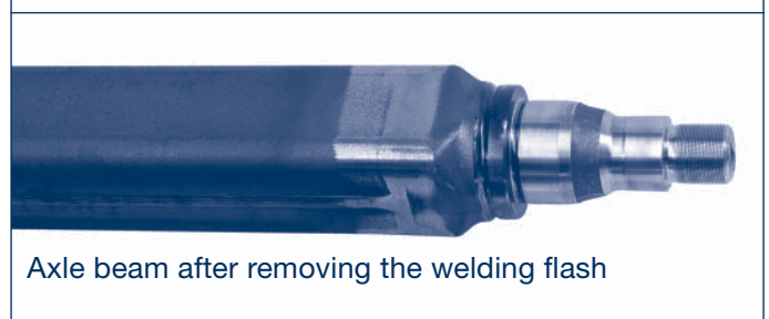
Axle beam after flash butt-welding
